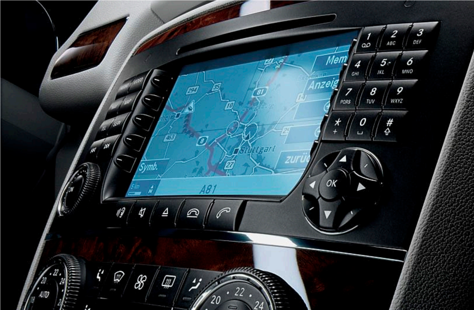
COMAND APS with its clearly legible 6.5-inch colour display
